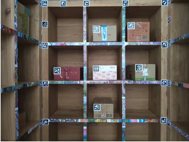
Fig. 4. The cargo shelves tagged with AprilTag markers.
