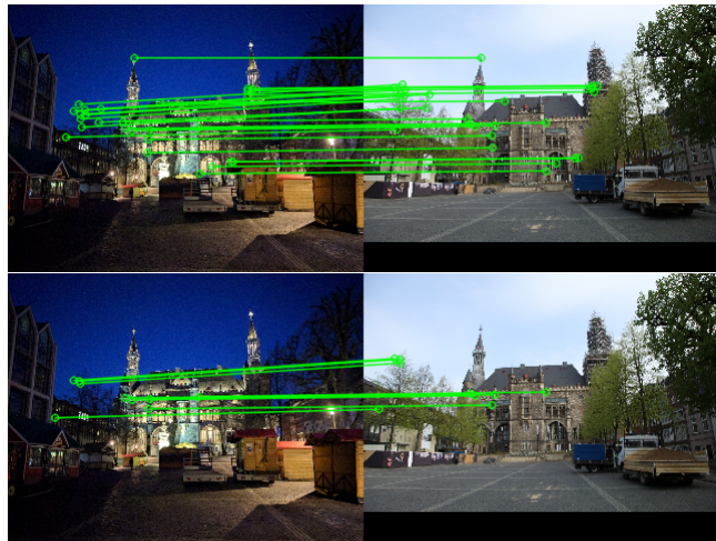
Figure 1: Comparison of the correct matches obtained by BGNet (the top row) and mutual check (the bottom row). On each row, the left is the query image, and the right is the retrieved nearest database image. All the correctly matched 3D points are projected onto this database image and the projections beyond the border are not displayed.
