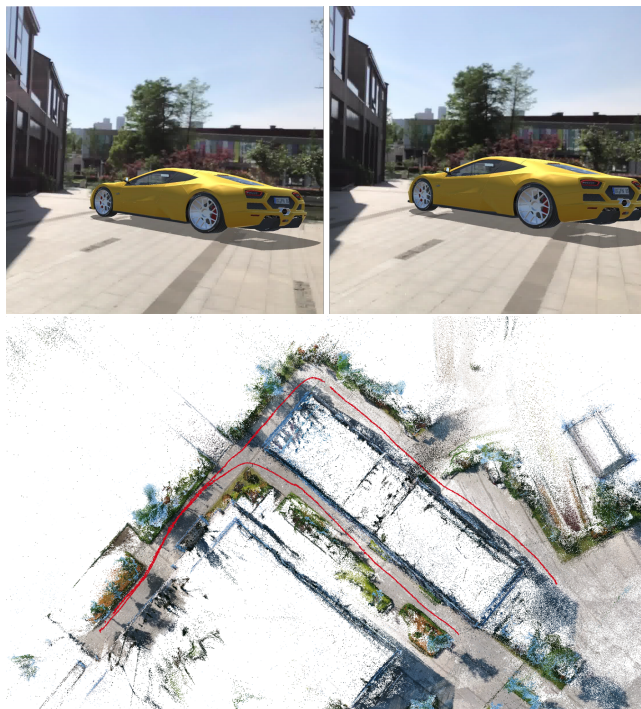
Figure 10: Visual localization for AR application. Top: two selected augmented frames. Bottom: the recovered camera trajectory superimposed in the offline 3D map recovered by SfM.
